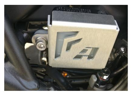
After 5 hours of riding, or 100 miles, check all the fasteners on the assembly to ensure they are tightened to spec.
