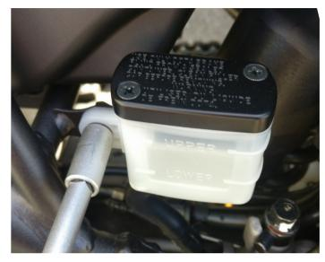
Use 8mm socket to remove the screw holding the rear brake reservoir in place.
