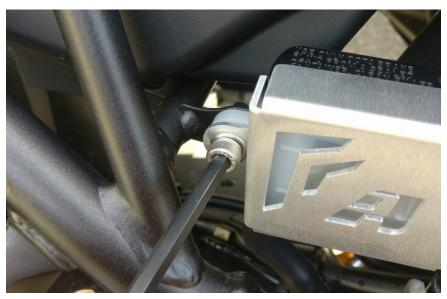
② Use 4mm allen tool with M6 cap head screw and washer to reinstall the reservoir guard.
